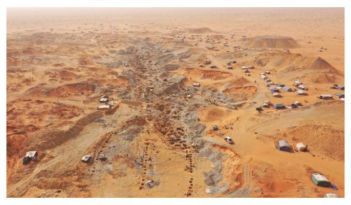
Figure 8: Wide Arial View of Illegal ASM gold extraction shafts at Zoerat Region
