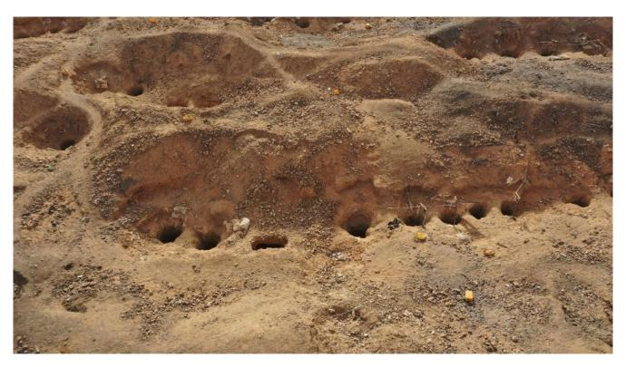
Figure 7: Close View of Illegal ASM gold extraction shafts at Zoerat Region
