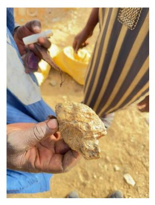
Figure 10: The quartz-rock containing gold
